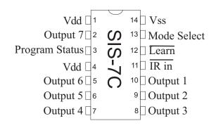
Vdd (with respect to Vss): 2-5.5V Provides up to 25 mA per Output pin Package: 300mil wide Plastic DIP IR in from IR module: No signal = Vdd, Pulses = Vss IR code is stored in non-volatile, re-programmable memory. Logic levels of Outputs 1-7 on power up: Vss (low)
